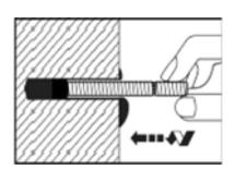
Push the threaded rod into the anchor hole while turning it slightly to ensure good distribution of the adhesive until the anchoring depth is reached.
