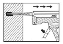
Start at the bottom or at the back of the cleaned anchor hole and fill the hole up to about one third with adhesive. Slowly pull back the nozzle as the hole fills to prevent air pockets from forming.
