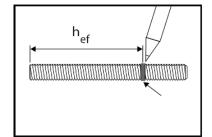
Before inserting the threaded rod into the drilled hole, mark the anchoring depth specified in the drawing on the threaded rods. Check the drill hole depth and the mobility of the threaded rod.
