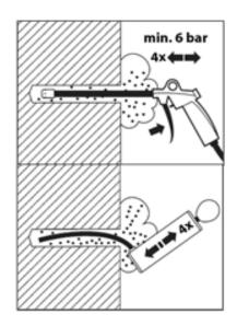
Cleaning with compressed air: Starting from the bottom or background of the borehole, blow out the borehole at least 4 times with compressed air (min. 6 bar).
