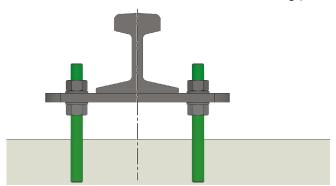
2. Place the clamps and mount the rail to the mounting plate using the clamping screws and clamping nuts.
