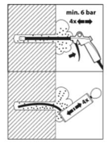
Caution! Standing water in the drill hole must be removed before cleaning!
