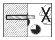
Allow the adhesive to cure for the specified time before applying a load or torque. Do not move or load the threaded rod until the special adhesive has fully cured.
