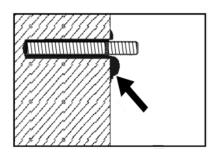
Make sure that the threaded rod is properly seated and that excess special adhesive is visible at the edge of the hole. If these requirements are not met, the application must be repeated from step 5 before the curing time is complete.
