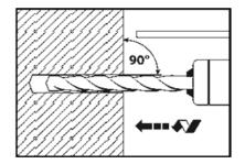
Use a hammer drill to drill a hole in the anchoring base in the size and anchoring depth (specified by the planner) required for the selected anchor size (see 3.2.2). In the event of drilling failure, fill the drill hole with mortar.
